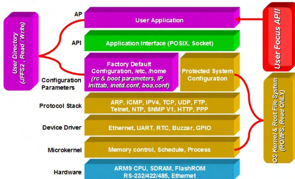
The EM-1240-LX's Flash ROM is divided into smaller partitions, including the Boot Loader, Linux Kernel & Root (/) File System Image, and User Directory partitions.
